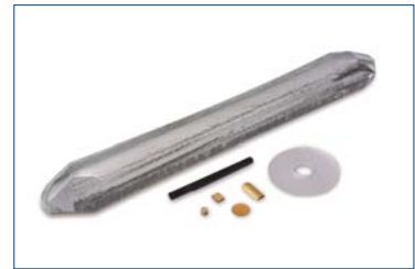
Quartz crystal used in piezoelectric sensors
